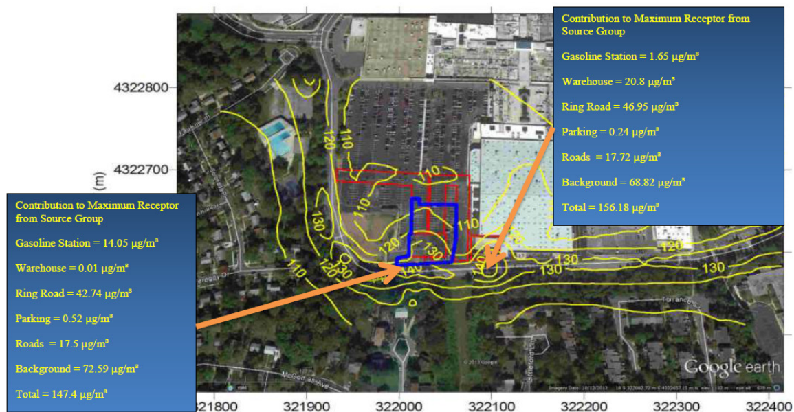
Figure 2: Stage 2 Predicted 98th Percentile Daily 1-Hour Maximum NO 2 Concentrations (µg/m 3 ) For All Sources Using Urban Dispersion, the OLM Method, and Hourly Concurrent Background (2006-2010) NAAQS = 190 µg/m 3 [MAX = 156 µg/m 3 at 322098X, 4322573Y] 62
